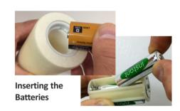
After the battery option is chosen, insert the batteries or battery caddy by pushing the end cap gently in and twisting anti-clockwise to release.
